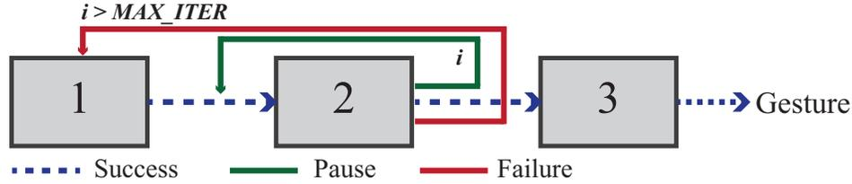
Figure 3: Execution process of three poses of a gesture and their states.
